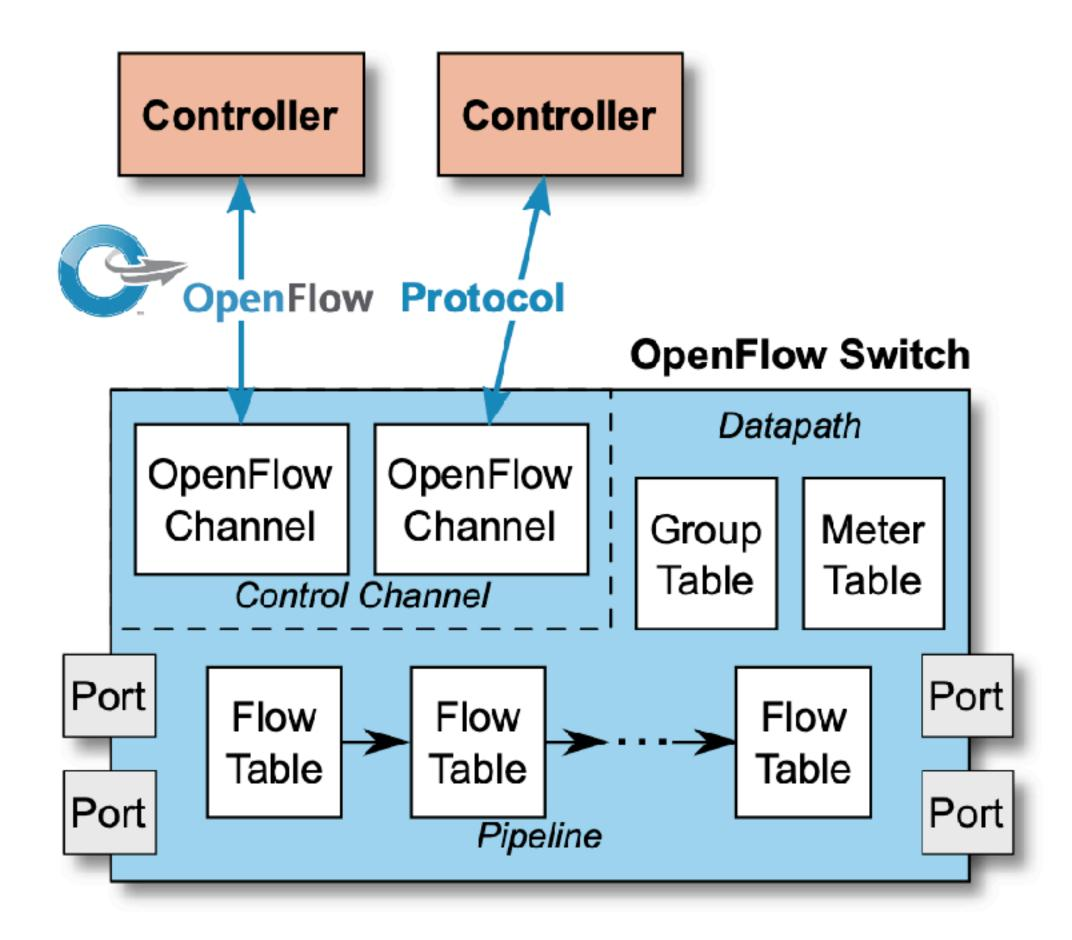
Figure 1: Main components of an OpenFlow switch.
