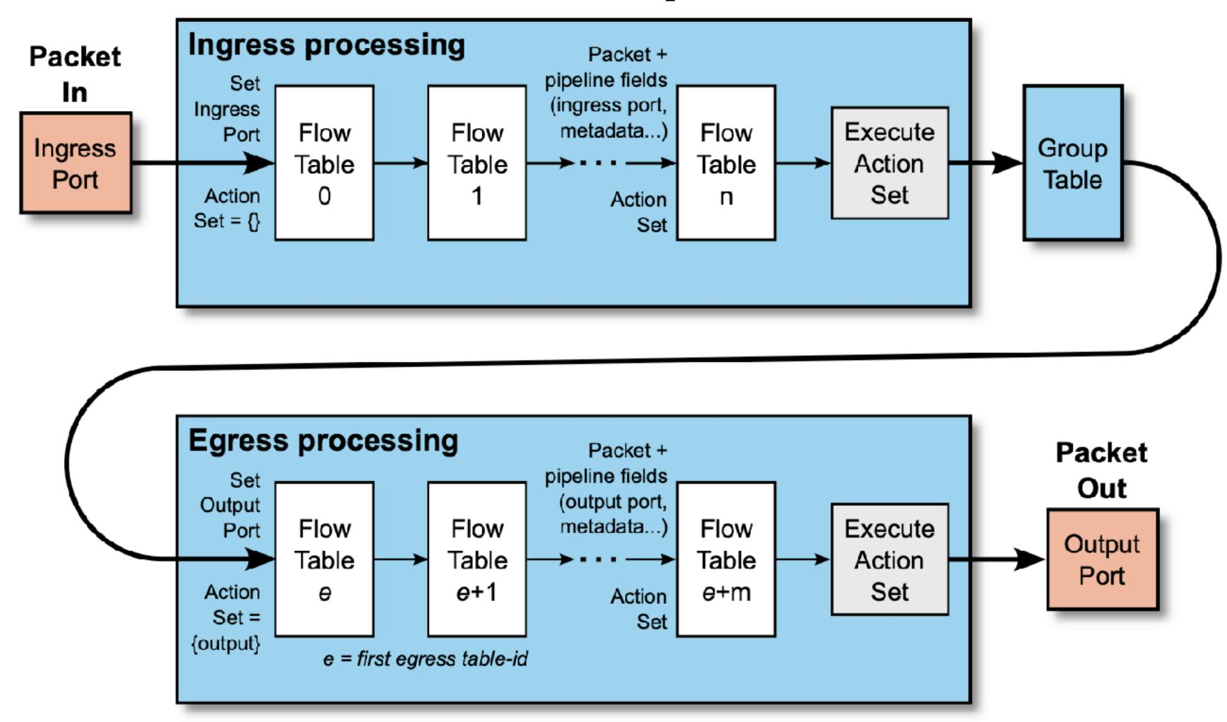
Figure 2: Packet flow through the processing pipeline.
